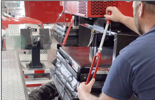
STEP 2.2: Hook turnbuckle (side B) into streetside unit tie-down, turn bar to right until tight.
