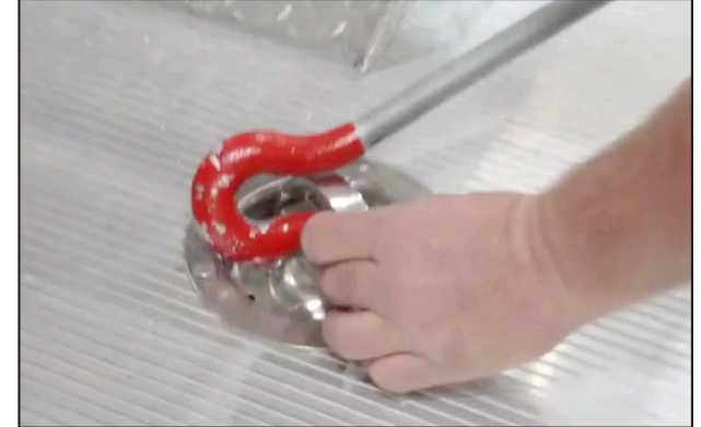
STEP 2.3: Hook second turnbuckle (side A) into curbside floor hook.
